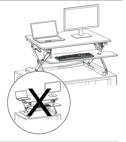
Prior to removing equipment from the CASSIOPEIA the work surface should be raised to the maximum elevation.
