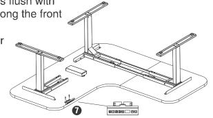
L. Connect the Wires as per the diagram below. Use the adhesive-backed Cable Clips (Part #13) to secure the Connecting Wires, so they don't sag.
